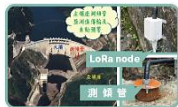
大壩監測儀器傳輸 Dam monitoring instrument transmission
